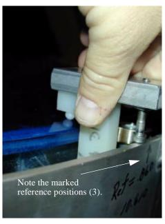
erly, this tool simultaneously touches the mirror surface and the top of the cell wall. In addition, the tool is pushed up against the sides of the mirror front and back plates. Height should be adjusted at 3 reference positions to within  $\pm -0.010$ -inch.
