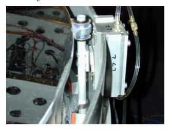
rod to give rough alignment with the actuator piston--then clamp.
