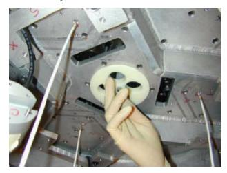
The height of the mirror is adjusted relative to datum A of the cell by using the mirror height tool at the 3 reference positions that are marked on the side of the cell. When inserted prop-
