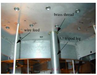
pod base off the platform because the brass thread binds with the clearance hole! Make sure to check hardpoint flexure clearance during this process. While continuing to lift the cell, screw nut (at base of tripod leg) onto the brass thread. When cell is lifted, the brass thread
