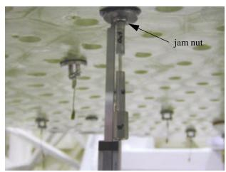
and use jam nut when length is correct. Do NOT bend flexures.
