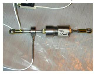
cell are labelled. They have integral tension/compression breakaways, so that they become "soft" when 15-lbs of force is applied to them. On both rod ends, there are spacer washers epoxied to each side of the spherical bearing. Take care to keep these intact.
