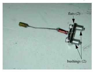
must be mated with the appropriate axial puck (already glued onto the mirror backplate). Note the two spacer bushings and the flat surfaces oriented toward the bolt heads.
