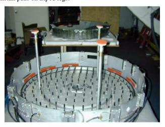
With 3 people each using both hands on mirror backplate, move mirror onto tripod taking care to align mirror and cell North orientations. Mirror backplate is marked with the pad
