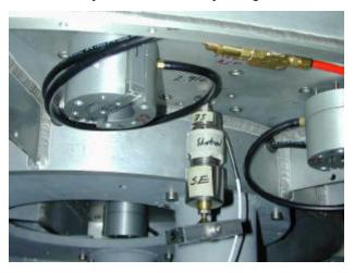
electrical cable coming out of the load cell interferes with the circular flange in the cell -- carefully handle flexure while screwing hardpoint on. Also, apply torque only to load cell body. Slightly tighten load cell against flexure nut.
