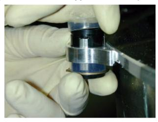
bearing pad, attach lower snap ring and clear bushing. Insert into bearing pad. Attach upper clear bushing, and *carefully* attach final top snap ring (not shown in this picture). Take care not to stress the bearing pad connection to the mirror or to let the snap ring launch onto the mirror surface.
