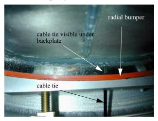
bumpers are directly under the mirror sidewall, so some care must be taken to push the tie in properly and far enough. Verify clearance for all axial bumpers. If adjustment is necessary, the radial bumper above it must be backed away from the mirror edge to allow access to the axial bumper brackets. This is a
