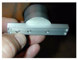
Install it onto the hanger ends using the 4 screws with 242 loctite.
