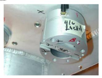
NOTES: Once assembled, grab the hanger with gentle force and make sure it has unrestricted clearance to go up and down by 1 or 2 mm each way. Do NOT assemble in a way that tensions the axial wire rope, because you could pull the puck off of the mirror backplate. In this same spirit, be very careful making mirror height adjustments henceforth. Raising the mirror height relative to the cell could tension the wire ropes!
