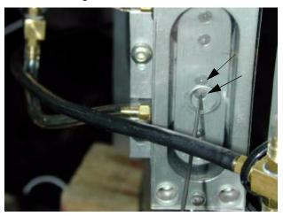
In addition to the short wire for L1, install the tangent arm connection onto this rod.
