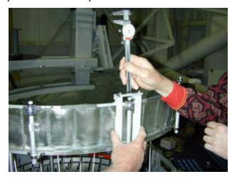
tool is shown in the photo (mirror is above cell for clarity). The tool must contact the top and bottom edge of the mirror and the balls on the surface of the mirror.
