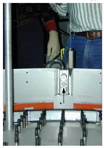
attached to the mirror to L7. When the mirror is properly clocked, the plumb point will be centered on the 3 ball bearings (arrow-mirror clocking is in error in this photo). Similarly, the plumb line off of the north mirror bearing pads to the L1 actuator will go through the center of the wire hole in that actuator body. Iteratively adjust centration and clocking by gently moving the mirror on the tripod legs as needed.
