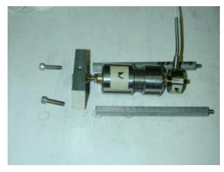
sponding labels on the cell plate. Each hardpoint has integral compession and tension breakaways that activate at 15-lbs.
