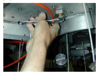
Check all the radial bumpers to insure they have a uniform clearance of about 0.040 to 0.05-inch from the edge of the mirror backplate. Adjustments are provided by the jam nut assemblies outside the cell OD.
