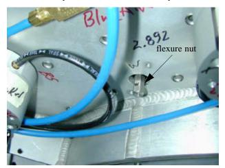
Locate the 3 axial hardpoint assemblies and attachment hardware. Each hardpoint is marked W, NE, or SE with corre-
