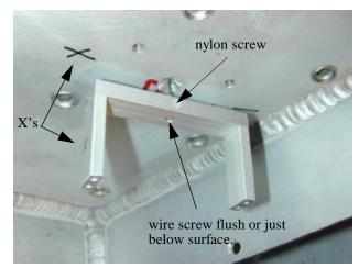
each hanger on until both of these conditions are met: 1) The "X" on the hanger and cellplate line up, and 2) the nearest revolution where the wire screw is flush or doesn't protrude from the lower surface of the hanger. It's important that the wire screw NOT protrude since the screw would limit actuator
