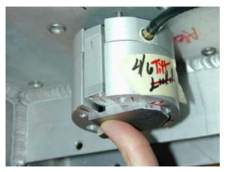
bottom as shown. Gently pull on hangar with a pound or two of force (taking care not to tilt the hangar). The lower surface of the crossbar should just touch the gauge. If there is more than 0.010-inch of gap or if the gauge is pushed away from the housing bottom by the same amount, the piston of the actuator must be adjusted. This tool has a 0.125-inch step and positions the hanger so it can move +/-1/8-inch during normal operation.
