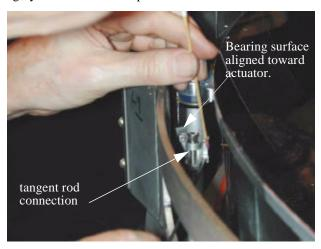
After installation and tightening, use penetrating loctite (we used 222) on the clamp screws holding the hardware onto the rod as shown in this picture.
