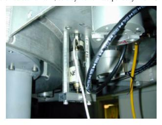
screw the two halves of the hardpoint breakaway against each other (large central thread). If the hardpoint was carefully removed, adjustment should be unnecessary.
