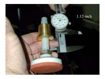
Install pads on tripod legs.
