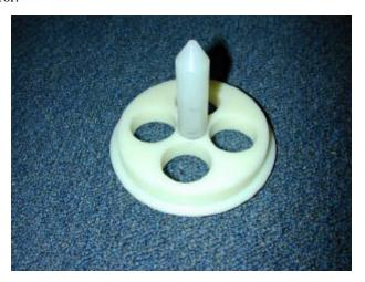
When the mirror is well centered, this tool is easily inserted and rotates freely.
