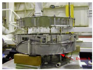
Take care to keep mirror centered and clocked properly as the cell is lifted. Also make certain that the tripod legs remain centered in their clearance holes in the cell plate. Use plumb bob as needed. Also, gently pull on wire feed-throughs to make sure axial cable doesn't buckle as cell is lifted.
