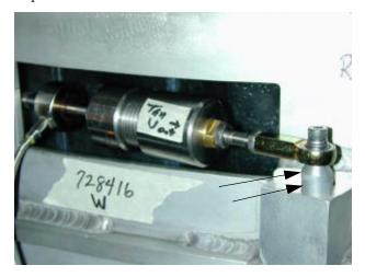
two spacer stackup (arrows) is underneath the rod end.
