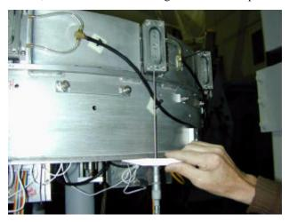
Set the depth micrometer to 6.325-inches, and adjust all lateral actuators to this position. This puts the line of force at 8.325-inches from datum A. Take care to uniformly align these to within +/-0.005 of each other. (NOTE: cg-calculations suggest that the cg is closer to datum A -- perhaps 6.310 or less -- but we were unable to adjust the actuators without hitting the cell midplane flange).
