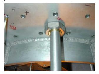
will extend below the nut by about 1/8-inch. There's a shoulder on the brass thread that WILL catch the clearance hole, so hopefully this was tapered per the note earlier. In practice, we had difficulty tightening these nuts, and ended up putting a stackup of 3 thick washers between the cell and nut.
