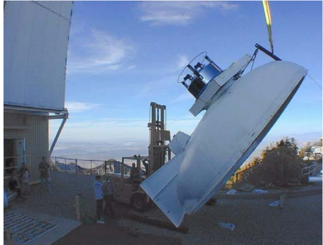
Figure 14. The vacuum head is tilted to vertical.
