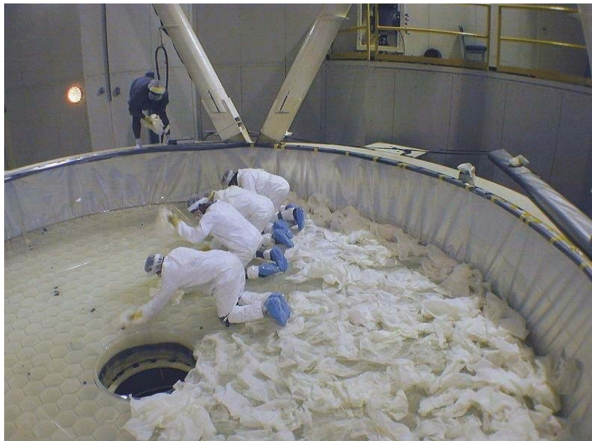
Figure 13. The surface receives a final wipe with very pure isopropanol.
