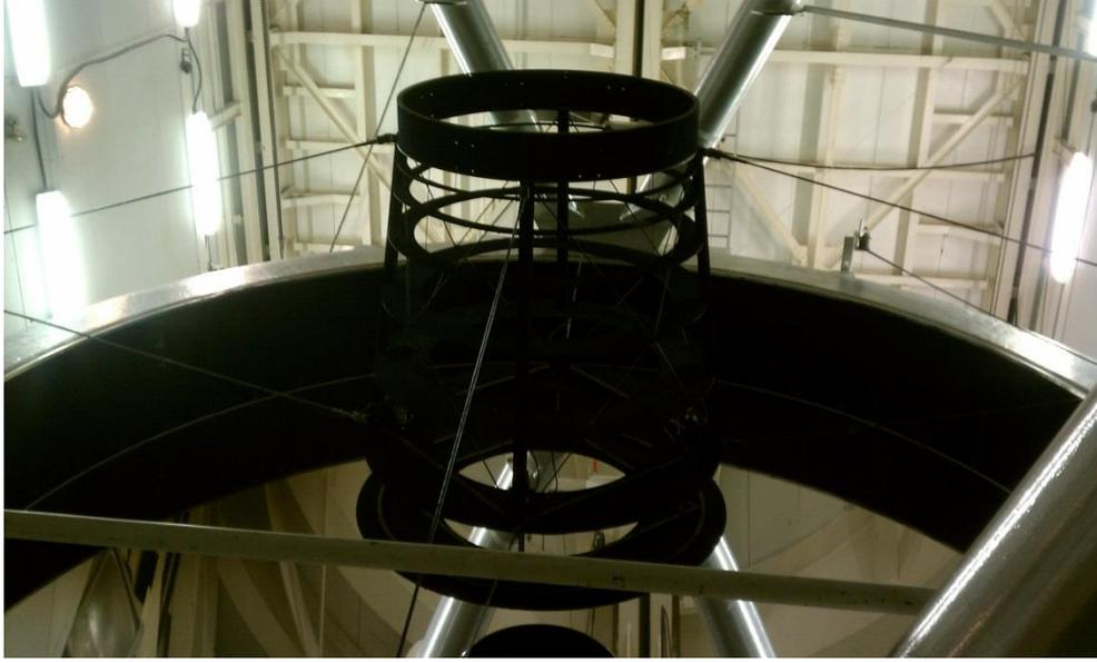
Figure 1. Mid-baffle extended at zenith.
