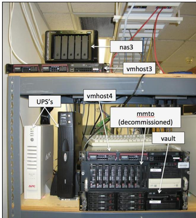
Figure 9. VM host computers, NAS boxes, and uninterruptible power supplies (UPS's) on the 3rd floor of Steward Observatory, on the campus of the University of Arizona. See text for additional details.
