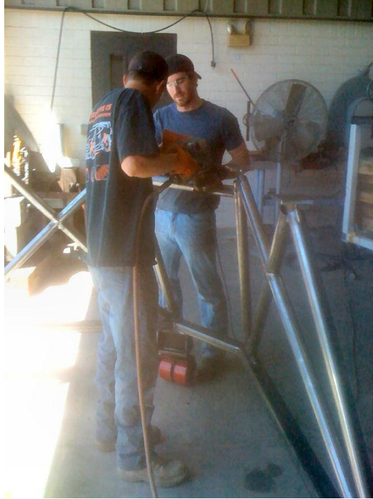
Fig 7. Fabrication of cart for LGS topbox.
