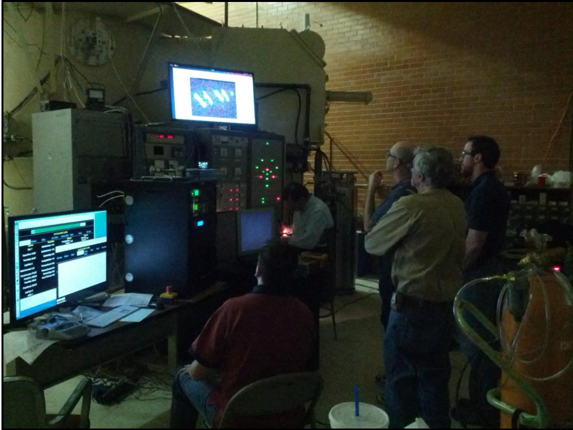
Figure 3. Large chamber testing at the Sunnyside facility. Shown from left to right are: R. Ortiz, G. Rosenbaum (in background), D. Clark, J.T. Williams, and J. Di Miceli. The aluminization software GUIs are shown in the lower left monitor. A close-up of the glowing filaments is shown on the monitor in the upper center of the photo. As the temperature increases, these filaments become white-hot. Control is automated during the tests. Staff mostly watches the monitors as the automated aluminization process proceeds, as the majority of the work is in preparation for the test.
