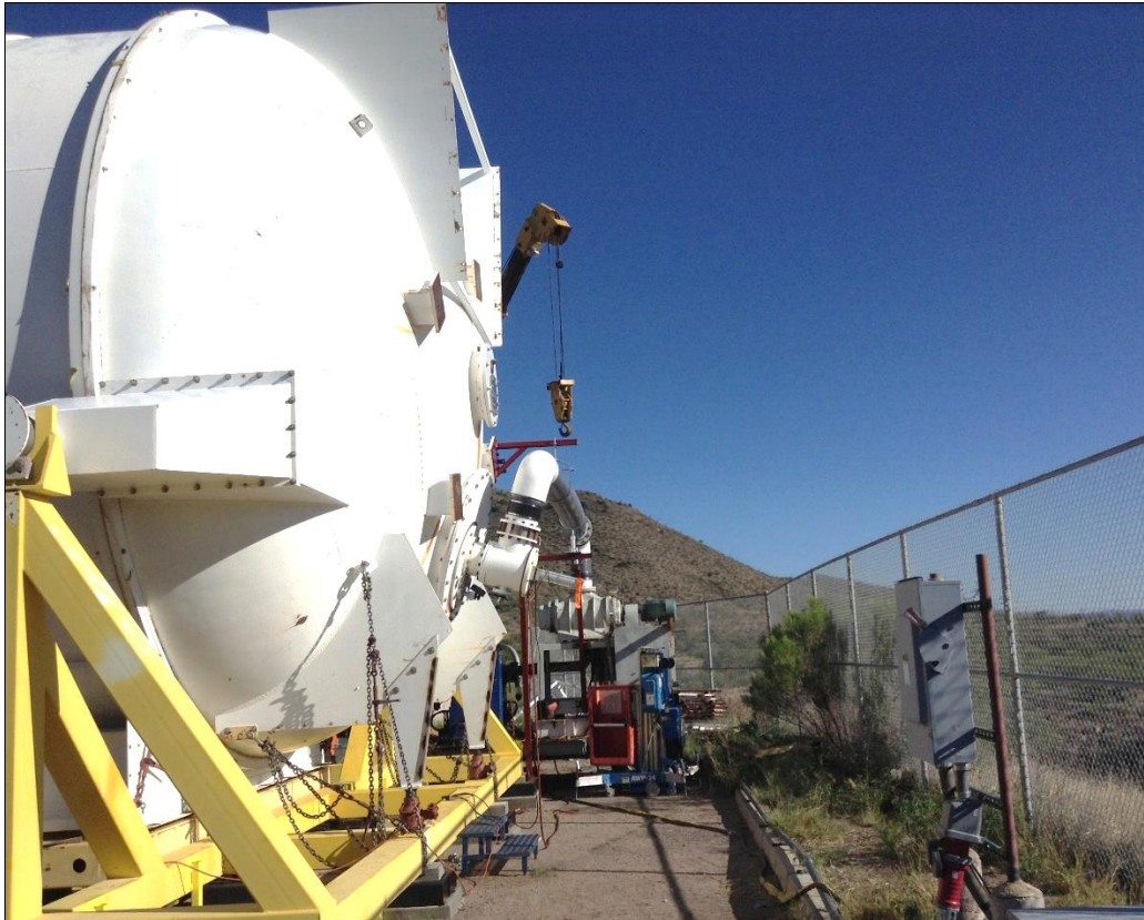
Figure 3. The roughing line is shown connected to the rear bell jar and pumping trailer.
