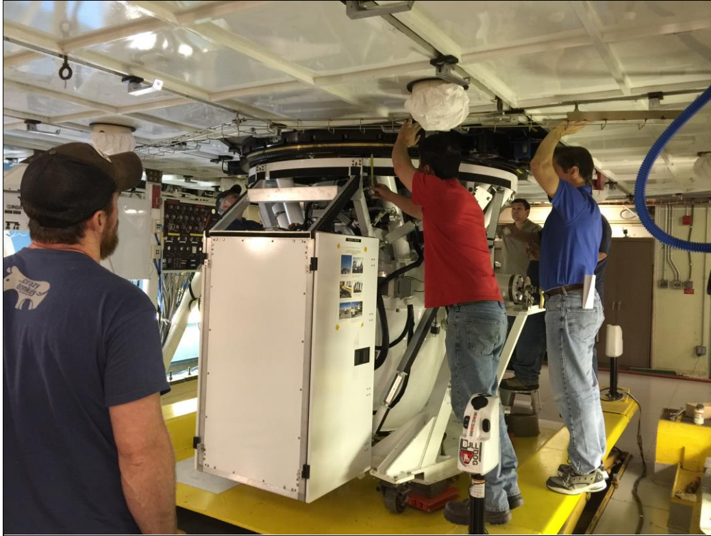
Figure 7. The MMIRS instrument being mounted on the telescope.
