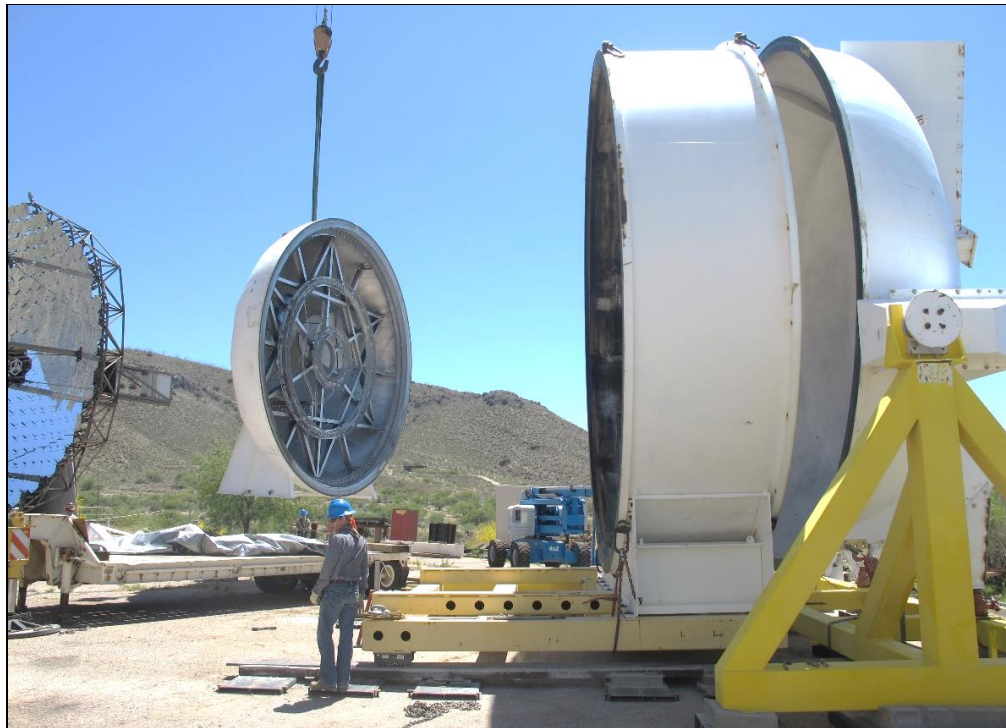
Figure 2. The bell jar is shown being moved into position on the bell jar cart.
