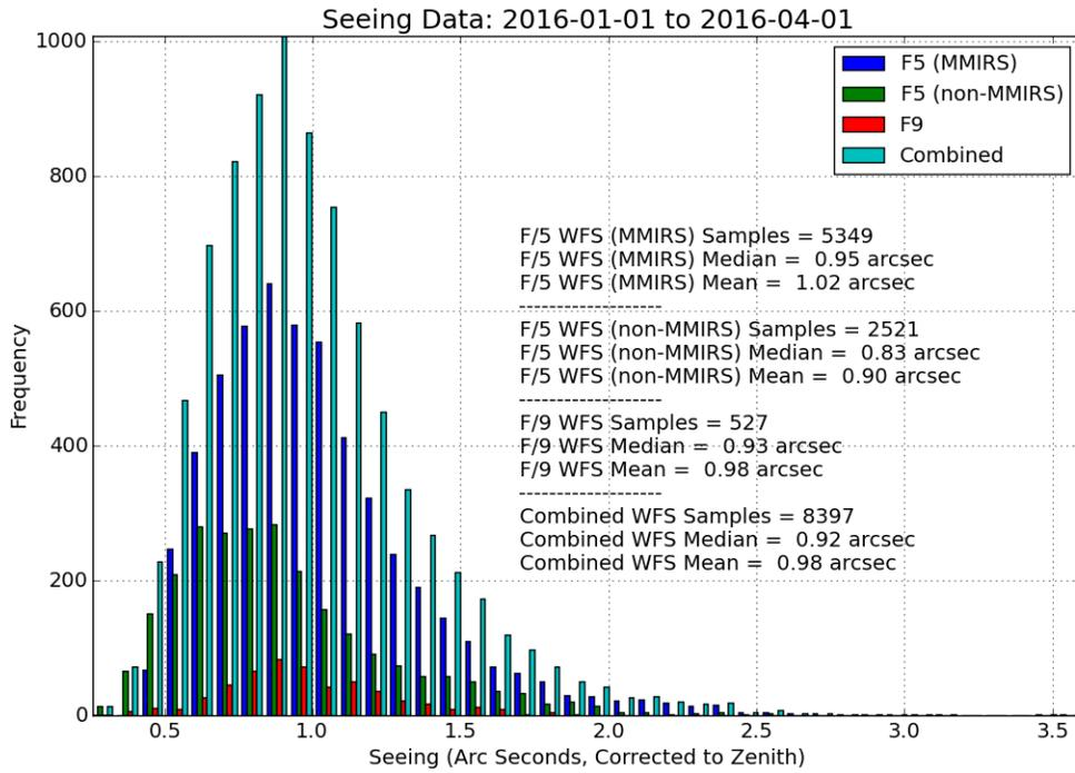
Figure 11. Histogram (with 0.1 arcsec bins) of derived seeing values for the f/5 (MMIRS and non-MMIRS) and f/9 WFSs from January through March 2016. Seeing values are corrected to zenith. The median f/5 MMIRS seeing is 0.95 arcsec and f/5 non-MMIRS seeing is 0.83 arcsec while the median f/9 seeing is 0.93 arcsec. A combined median seeing value of 0.92 arcsec is found for the total 8397 WFS measurements made during this period.
