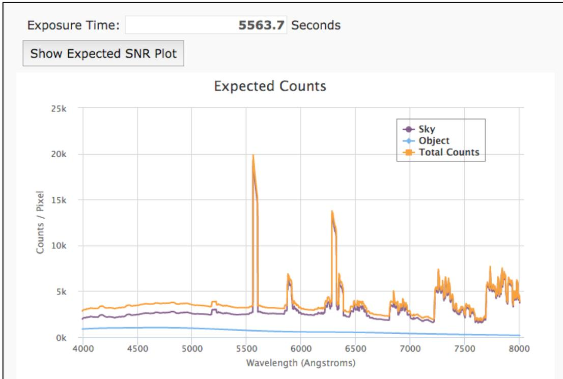
Figure 8. Expected counts per pixel for the total spectrum (orange), sky (purple), and object (blue) for a flat-spectrum 21 magnitude source observed for 5563 seconds. The user can understand the relative contribution of major sky features on their target.
