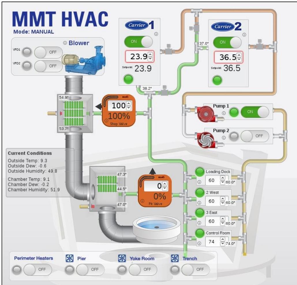
Figure 6. Modifications were made to the HVAC control GUI to include the perimeter heaters and the pier, yoke room, and trench fans. A separate control GUI for these fans is no longer needed.
