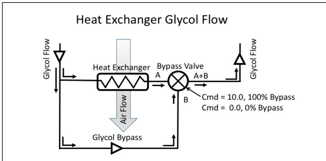
Figure 5. Schematic diagram of glycol flow through the shop and pit heat exchangers. A Belimo bypass valve was installed for each heat exchanger during the HVAC upgrade that allows glycol to flow either through the heat exchanger or around (*i.e.*, bypass) the heat exchanger.
