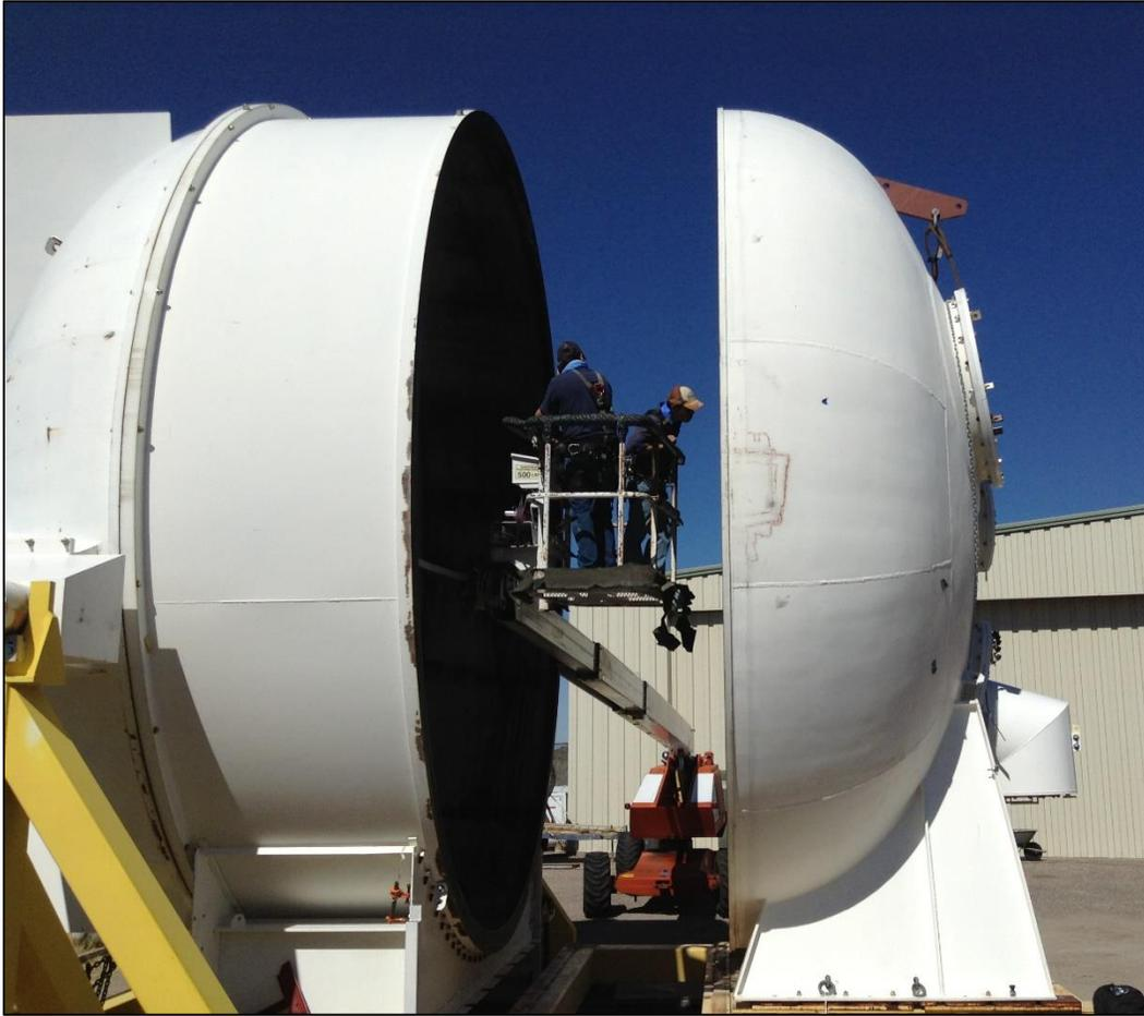
Figure 3. R. Ortiz and C. Chang positioning the lift to start filament installation.
