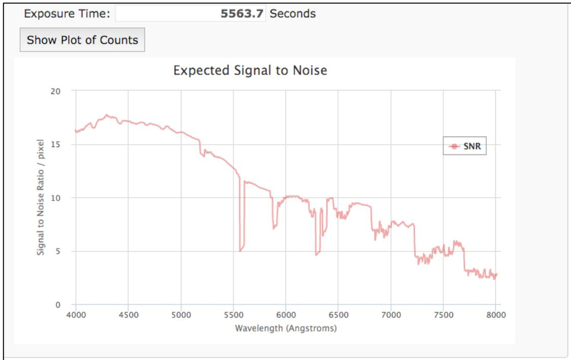
Figure 7. Expected signal-to-noise (per pixel) for an R=21 AB source observed for 5563 seconds (the needed exposure time to reach a mean S/N of 10).
