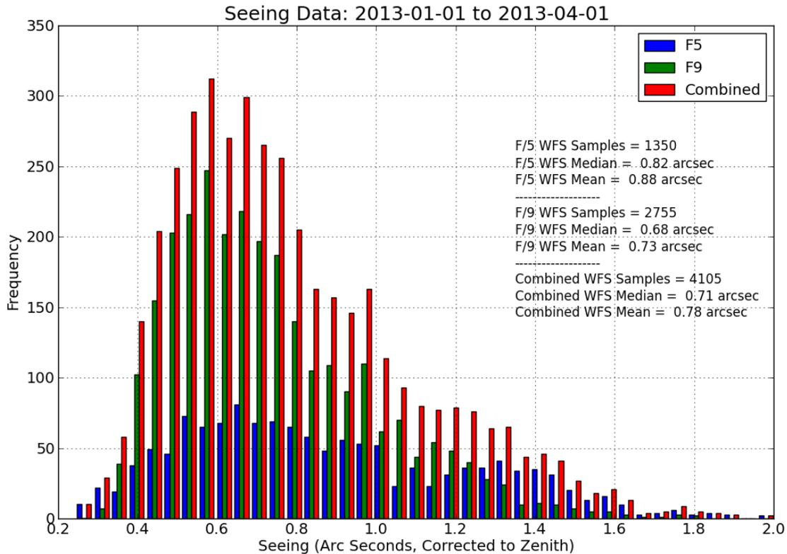
Figure 13. Histogram (with 0.1 arcsec bins) of derived seeing values from the f/5 and f/9 WFS for January through March, 2013. Seeing values are corrected to zenith. Median f/5 seeing is 0.82 arcsec while the median f/9 seeing is 0.68 arcsec. A combined (f/5+f/9) median seeing value of 0.71 arc-sec is found for the 4,105 WFS measurements made during this period.
