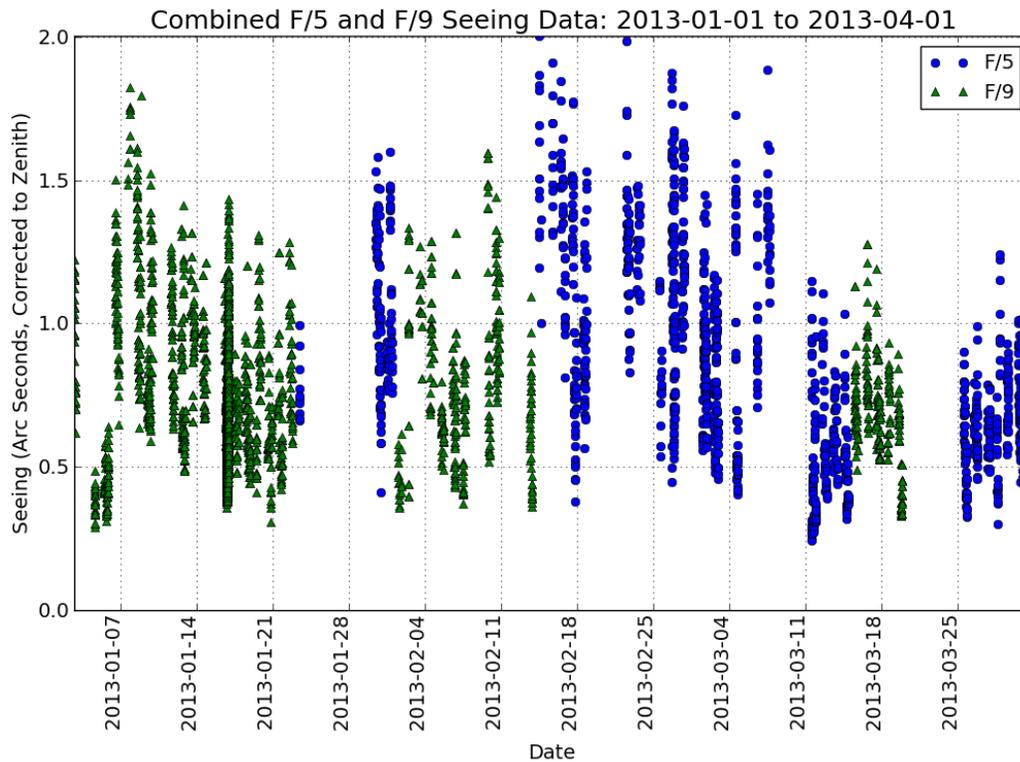
Figure 12. Derived seeing from the f/5 and f/9 WFS for January through March, 2013. Seeing values are corrected to zenith. f/5 seeing values are shown in blue while f/9 values are in green. An overall median seeing of 0.71 arc-sec is found for the 4,105 WFS measurements made during this period.
