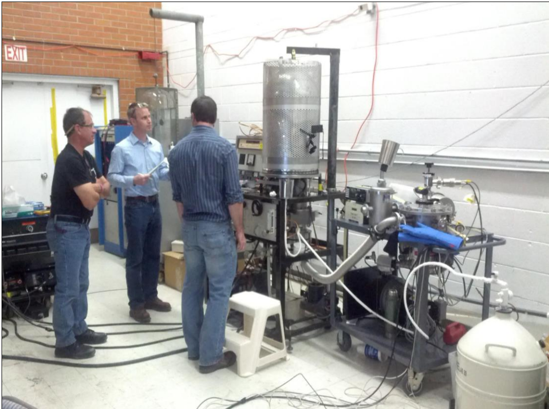
Figure 2. Testing with the small vacuum chamber at the Sunnyside test facility during March 2014. B. Comisso, W. Goble, and J. Di Miceli are shown, left to right. This small test chamber is used for coating small surfaces, such as test slides. Because of its rapid turn-around, 8-10 tests can be done in a single day.
