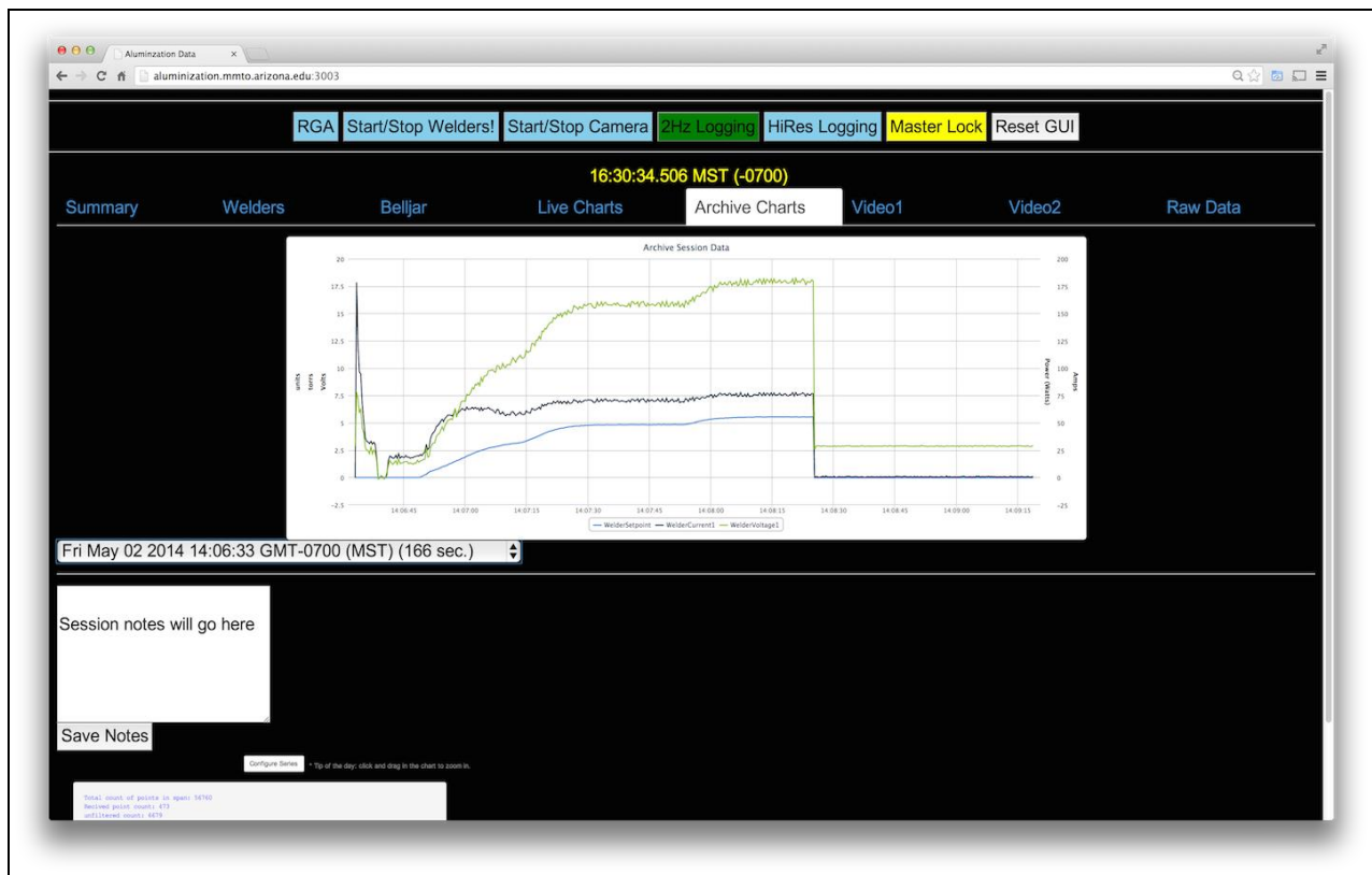
Figure 3. A sample of aluminization data collected using the ‘archive charts’ plotting tool. Any of the tests performed can be selected from a relational database, and over 100 parameters related to each test can be plotted versus time. This GUI has been particularly useful as a “quick look” visualization tool during testing.
