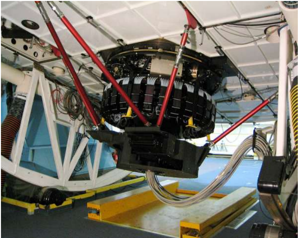
The Hectospec/Hectochelle fiber positioner and derotator mounted at the Cassegrain focus, prior to installing the fibers. (Image by D. Fabricant.)
