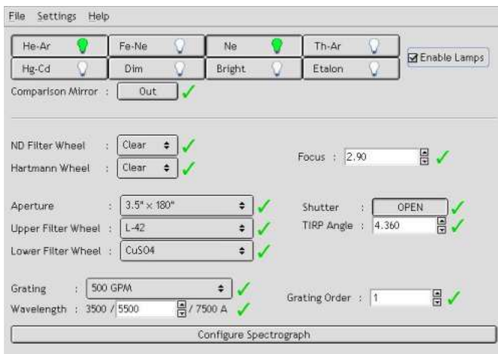
Figure 7: Layout of current GUI for controlling the spectrographs and topbox lamps.
