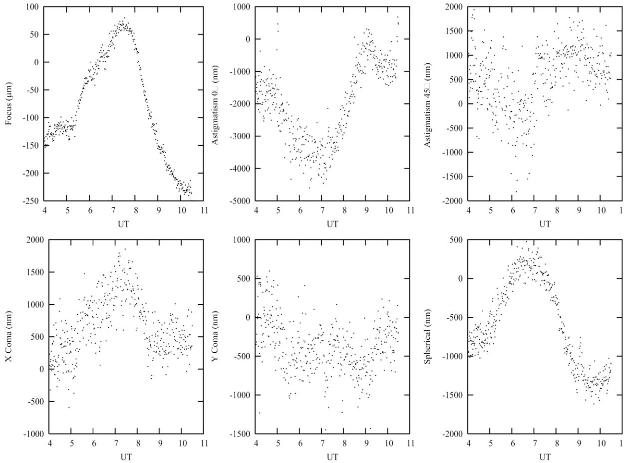
Figure 5: Results of wavefront measurements over the same period of time shown in Figure 3. The large scatter in the data is due to the fairly poor seeing conditions ( $\sim 1.5''$ ) during the time the data were taken. In spite of this, the variations in focus, spherical aberration, and 0-degree astigmatism are clearly seen.
