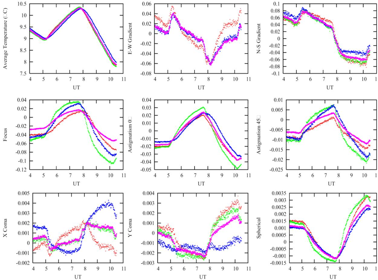
Figure 4: Results of Zernike polynomial fits to the temperature structure of the primary mirror over the course of the night of November 21, 2005. In all plots the red data corresponds to the front plate, green to the mid plate, blue to the back plate, and magenta to the average temperature. The temperatures all come from the cell's E-series thermocouples.
