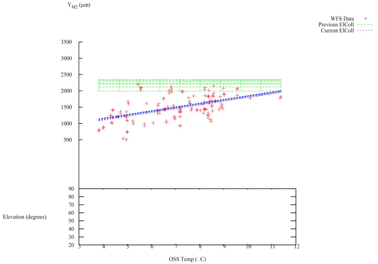
Figure 2: Known good M2 Y positions as logged by the WFS (red crosses) during the last two weeks of December 2005 plotted with EIColl fits determined from dedicated observations during November 2005 engineering time (green dashes) and by fitting a model to the WFS data (blue dashes). The data are projected to most clearly show the temperature dependence seen in the December WFS data.
